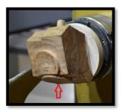
In this case, it is still critical that the top jaw and tailstock are centred on the draft hole pencil line.
