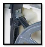
Dust/pitch buildup on the wheels will affect tracking and produce vibration. While a tire brush will not prevent this, it will help to minimize the buildup. While you could configure your own system using a stiff brush, the cost of a manufactured one is relatively low (LV: \$9.50)
