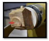
For this orientation, Emma strongly encouraged the use of a tenon to hold the blank (left: arrow). Given the amount of wood which needs to be removed and the offset stem housing, this is a far safer option.
