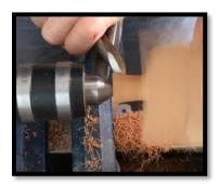
With the tailstock engaged, the stem housing is turned to its final thickness and then sanded.
