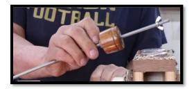
With a wooden washer and nut on one end of the draw bar, it is inserted into the headstock and screwed into the end of the chuck. The nut is then cinched up to hold the chuck securely in the headstock spindle.
