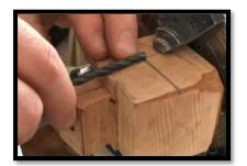
The next step is to drill the draft hole using a 5/16" bit. The depth of the drilling should be set so that the outer wings of the flute meet the centre of the tobacco chamber (left). Given the length of this bit and its tendency to wander, using a machinist's drill bit is highly recommended.
