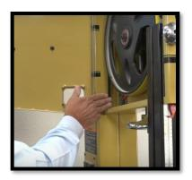
Rather than checking tension at the table, he recommends opening the top wheel cover and checking the blade tension at the "back" of the saw.
