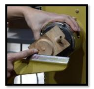
She first uses a parting tool and gouge to form a short portion of the outside diameter (left) and then hollows the bowl portion using a negative rake scraper. She continues until the draft hole is located at the bottom of the chamber.
