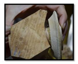
A bead of hot melt glue is applied to the waste block to secure the blank and the tail stock is engaged to provide the proper orientation.
