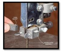
Cool blocks are not only the cheapest, but they also allow you to position the leading edge right at the deepest part of the gullet to provide maximum support.
