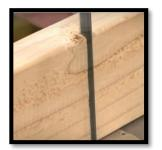
A more accurate method is to make a shallow face cut on a piece of 2x4 or 2x6, flip the board around and try to slide the back of the blade into the cut slot. If it enters smoothly the table is square to the blade.
