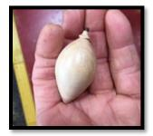
He had mistakenly believed that he was using waxed nylon string! As you can see in the photo, the unwaxed string quickly burned through the narrow cylinder.
