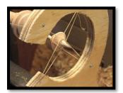
However, as the turning proceeds, it becomes necessary to provide support at the narrow spindle areas. For this purpose, a set of string steady rests are required in which the piece is stabilised by string as opposed to wheels.
