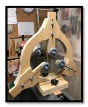
Further to the article in the February newsletter on Hollowing Tools, Alan Cusworth of the Greater Vancouver Woodturners Guild recently designed and built an impressive custom steady rest. You can find pictures and a detailed description of how to build it in the February edition of the Vancouver Guild's newsletter:
