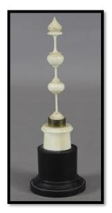
A *trembleur* (aka *wobbler*) consists of a series of small ornamental forms that are separated by very thin sections of consistent diameter. The name derives from the fact that the turning will vibrate or "tremble" at the slightest touch.
