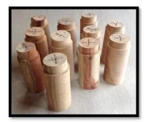
The blanks are turned between centres and measure 4'' in total length by 1 3/4" in diameter with a 1/2" to 5/8" long tenon.
