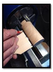
Using a spindle gouge, I turn the small end of the egg and a **small** portion of the large end to develop a smooth curve. I found that if I removed too much wood on the large end, the blank developed harmonics. The surface is then refined using a skewed negative rake scraper.
