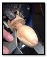
I then shape the large end, leaving a tenon about 5/8" in diameter with a groove between the tenon and the egg. (See diagram below) The groove allows me to sand right to the base of the curve.
