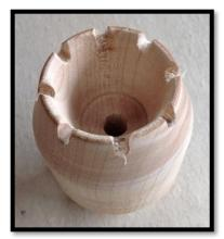
A series of "glue" slots are then cut in the rim of the chuck and a through hole is drilled in the centre to enable removing the egg using a leather-tipped dowel.
