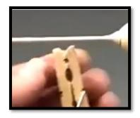
To minimize vibration, he uses a homemade steady rest which consists of a wooden clothespin glued to a piece of dowel. The clothespin has a hole drilled in it which matches the diameter of the stem (left) The dowel is set into a block of wood which has 4 rare earth magnets to secure it to the lathe ways.
