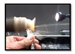
He then finishes turning the outside of the bowl using a light source to determine the thickness of the bowl.
