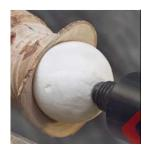
He slowly tightens the tailstock until it just barely moves the turning. Ensure that the "ball" does not rotate inside the turning.
