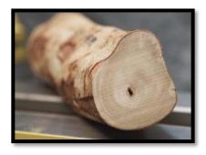
The most important requirement when mounting the blank between centres, is to avoid having any pith in the stem. Otherwise, it will break. Ensure that you offset the blank from the pith on the same side at each end.
