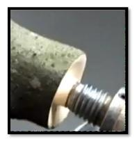
After squaring up the end, establish the rim and begin to hollow the bowl portion using a 3/8" bowl gouge. As the photo at left shows, you will not be able to go very deep since the live centre will be in the way.
