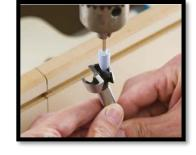
These bits can also be used in a rotary tool although I found it much harder to maintain a consistent honing angle.
