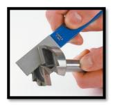
For all 4 types of bits, the chipper (bevel and face) is sharpened in the same manner. Most recommend using a 600-grit diamond paddle hone on both surfaces, taking care to ensure that you match the machined angle on the bevel.
