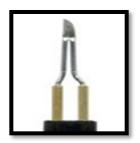
As most of my work consists of very fine burning, I use the extra-small knife (F14XS) which will burn 120 lines per inch.
