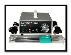
All 4 manufacturers offer dual port machines. While this enables one to have two pens plugged in, it is important to note that only one of these will be hot at any one time.
