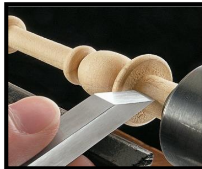
Peeling/Parting cuts (Straight on)
