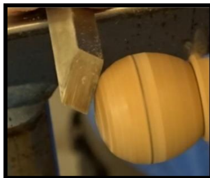
Shear scraping (Centre of bevel at 45-degree angle)
