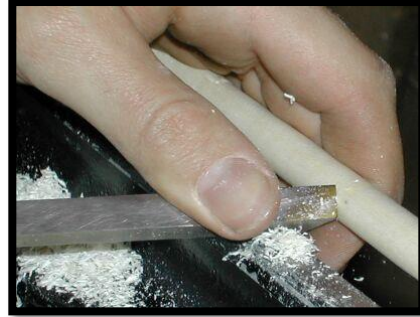
Peeling/Parting cuts (Straight on)
