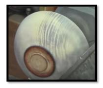
He uses a hot air gun to dry the dye and then begins to sand off this coat. He indicated that there is no right answer as to how much base colour to remove. However, consistent pressure and lathe speed is crucial to ensure an even removal of the dye.
