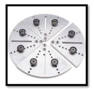
While Martin uses a vacuum chuck, he noted that if you do not have one, you could use Cole Jaws (left) or a custom-made friction drive (below).
