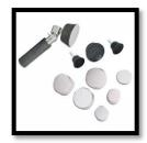
He typically begins at 120 grit and moves up to 400 grit. Any higher grit would fill the wood pores which could interfere with absorption of the dye. With each successive grit, he reverses the direction of the turning. However, unlike many other turners, he does not reverse the drill rotation when reversing the lathe direction which is likely attributable to his normal use of an inertia sander.
