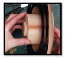
Whatever method you use, Martin emphasized the need to ensure that you have a dimple on the centre of the tenon/recess for alignment using the tailstock.
