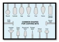
As the diagram shows, burrs come in a variety of shapes. While the best shape will obviously depend upon the nature of the carving, the most used shapes are the ball (round), cylinder and flame.
