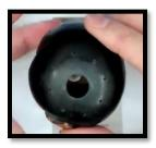
He has been able to find a kit from KMS tools which contains a much smaller diameter cap. In other cases, he simply discards the cap and drills holes in the "hair piece".
