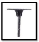
The disk is relatively firm, so he sands the outer edge to reduce thickness and increase flexibility. He then glues Velcro hook pads on the face for quick change using loop-backed sandpaper. He emphasizes the importance of using these discs at a slow speed (7,000 rpm) and with a light touch.
