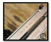
This tool makes it easier to maintain a parallel position and the indent lines (typically 25 and 30 degrees) assist in maintaining the required angle. More importantly, these guides position the file at the appropriate height on the cutting edge (approximately  $1/5^{th}$  of the file above the top plate) thereby avoiding the common problem of the file being set too low in the gullet.
