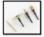
Sintered burrs are almost as durable as carbide burrs and can be sharpened with a diamond dressing stone. Most sources suggest that they will last 10 times that of plated burrs, a point which is reflected in their cost. Sintered burrs cost \$30 (KV Wood Carving Supplies) while plated burrs (from a reputable manufacturer) cost approximately US\$5 (MDI Woodcarvers)
