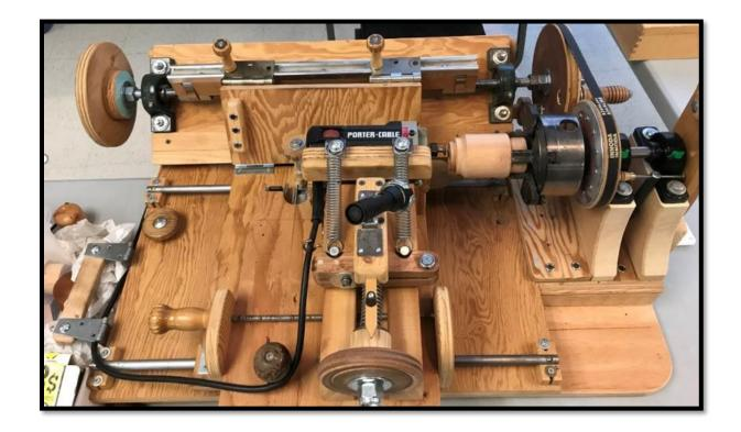
Most commercial jigs have the cutter mounted in the headstock of the lathe and use the tailstock to hold and advance the workpiece. Gil chose to install the cutter in a trim router and relies upon a series of threaded rods and stops to adjust the length and depth of the threads.
