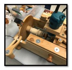
The number and location of the slots are determined using a pointer and the index wheel.
