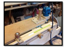
The top plate slides "fore and aft" with the amount of movement regulated by two locking knobs using the on-board measuring tape.
