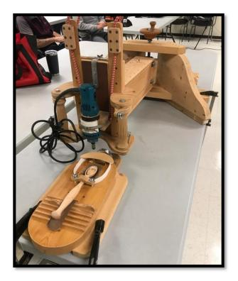
Gil built this jig to speed up the carving of the bowl portion of spoons. The spoons are turned with a round bowl and the top "half" is removed at the bandsaw.
