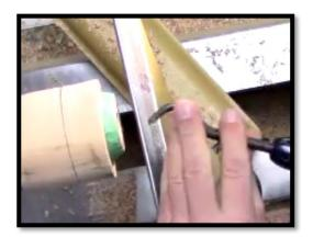
He then hollows the turning using a One-Way termite for the end grain and finishes the shoulder areas using a Hunter Full Swan tool with a carbide cutter.
