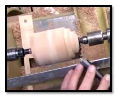
The blank(s) are then mounted between centres and a few dabs of hot glue are used to secure the orientation. Tenons are then turned on each end.
