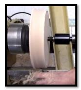
The outside of the blank is turned, and then he added a small bead at what will be the top of the cabinet.
