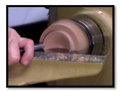
The top piece is then mounted and a tenon is turned to provide a relatively loose fit with the base.
