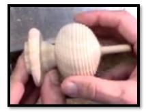
The widest part of the form is 2.5" and this should be located approximately 2 ¼" from the tailstock end. A light pencil mark is made at this point. The bottom of the form is turned to approximately 1.25" diameter.
