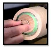
The bottom is then turned flush leaving a diameter greater than 1" for the plug. He creeps up on this for a tight fit.
