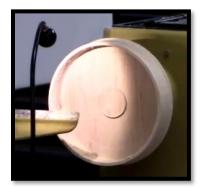
He then hollows the form to approximately 1/4" thickness at what will be the top of the cabinet. For reverse mounting, he turns a shallow tenon on the inside (left).
