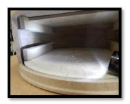
Kai first turns a piece which will be cut to form the Inside Arc of the drawer (see diagram above). This piece is 3/16'' - 1/4'' square.
