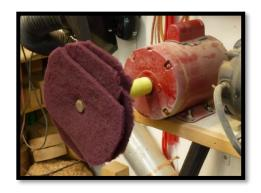
Tim mounts 4 pads on a threaded bolt with fender washers between each pad and a washer and nut on the end and then installs the assembly on a separate motor.
