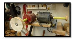
While he mounts these on separate motors (1725 rpm for 8" pads and 3450 for 4" pads), many turners opt to mount them on their lathe. For this, you will need a #2 morse taper adaptor (LV: \$15). As this will provide limited clearance from the headstock, many also purchase a 3" mandrel extension which will provide a total 6.75" reach. (LV: \$28).
