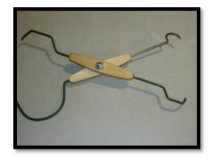
To measure wall thickness, he uses a homemade doubleended caliper.
