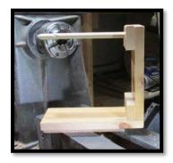
This is the jig that Graeme uses to measure the thickness of the bottom of a turned piece (and to avoid turning a funnel).
