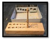
To accomplish this, he drilled a set of holes into a piece of hardwood and uses this template to determine the appropriate drill bit size. Simple but effective!
