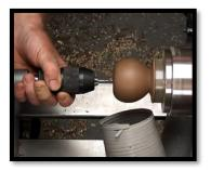
He applies a finish to the piece and then removes the blank from the chuck without parting it off.
