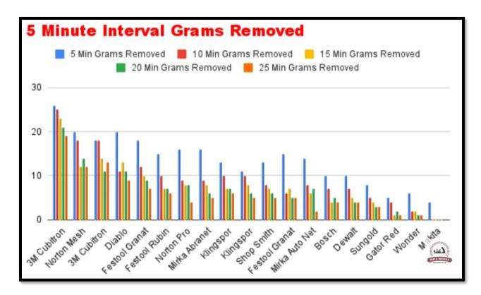
In the **5**<sup>th</sup> **interval**, the *3M Cubitron mesh* removed a total of 19 grams. This was matched only by the *Norton Mesh* and the *Diablo*, in their **1st interval**. Thereafter, the efficiency of these two as well as all others significantly declined. For example, while the *Norton Pro* and the *Mirka Auto Net* performed very well in the first 5 minutes (which boosted their overall "score"), they removed very little wood by the 5<sup>th</sup> interval.
