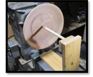
When the dowel is engaged with the turning, the distance between the masking tape and the front edge of the base indicates the thickness of the turning.
