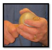
To accomplish this, he uses a set of fids. One has 4 hacksaw blades glued in lengthwise while the other one is wrapped in coarse sandpaper.
