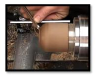
The blank is mounted in a chuck, and he uses a small bowl gouge with a fingernail grind to shape the top sides of the apple and the "indent" for the stem.
