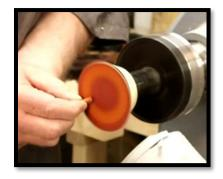
He then sands the top at an angle and secures it in the turning with a drop of glue.
