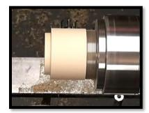
With the scrap mounted in the chuck, he turns a concave shape on the face matched to the size of the top of the apple. He then drills a screw hole in the centre.
