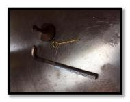
He bends over a short length of 20-gauge brass wire and mounts this in a hand vice. With the vice secured, he installs a nail with a 90-degree bend at the tip (left) in a drill and slowly twists/braids the wire.
