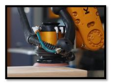
Each disc was tested for five 5-minute intervals on boards of red oak. The boards were weighed before and after each interval to determine the number of grams of wood removed. To determine the best value, the cost of each disc was divided by the total grams of wood removed to produce the cost of grams removed.
