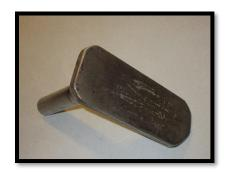
And, as he found it difficult to hold securely on a conventional tool rest, he uses a custom rest which has a large flat bearing surface.
