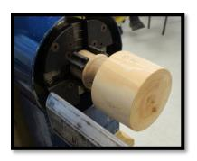
He begins with a small blank of Douglas Fir. To save wood, he drills and glues a small dowel which is then mounted in his spigot jaws.
