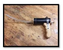
Prompted by an analysis of fireplace bellows, Gil made the "Puffer". He installed a flap valve inside a piece of ABS pipe which allows air to blow out but prevents air being pulled in.
