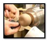
He sands the outside to 600 grit and with a Jacob's chuck in the tailstock, drills a 3/32" hole in the top for the stem.
