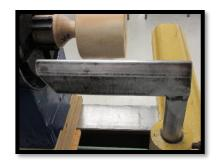
To clean up the surface he first uses a negative rake scraper. He has two of these in a skew shape for left, and right hand, scraping.
