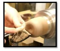
A skew is used as a negative rake scraper to blend the top surfaces.
