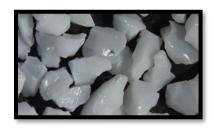
It has a seeded-gel ceramic abrasive with a stearate coating designed to minimize loading. While it does not have a mesh structure, the paper backing is latex-saturated, and fibre reinforced to provide strength and flexibility.
