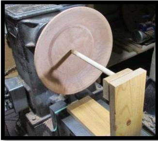
When the dowel is engaged with the turning, the distance between the masking tape and the front edge of the base indicates the thickness of the turning.
