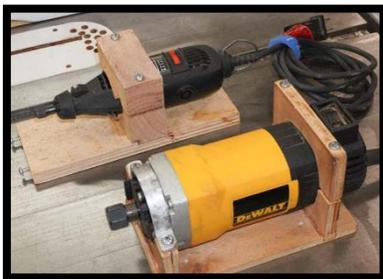
Wooden carriages range from the simple (left) to more complex rigs such as the one that Gil Heise made for integration into an XYZ platform (right).
