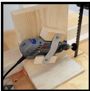
If you own a Dremel (or facsimile), you can use this jig to quickly sharpen your bandsaw blade using a cut-off disc.
