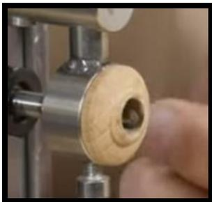
Accordingly, most jigs rely upon a "nose bushing" which rides on the surface of the turning. These can be made of wood, plastic, or, in the case of Mike's carriages, metal.
