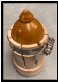
If turning an egg from a blank held in a chuck, one is faced with the challenge of finishing the end of the egg which was in the chuck. This jig enables Graeme Evans to quickly complete this task.
