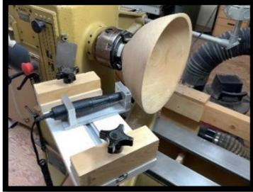
A track with adjustable stops can be added to limit the carriage's travel.
