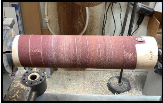
He made the drum by turning a cylinder and wrapping fabric-backed abrasive tightly around it. The ends are secured with screws and washers.
