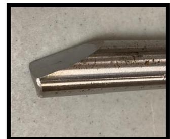
Used on their side so that the lower part of the edge is nearly vertical, they slice through the wood.
