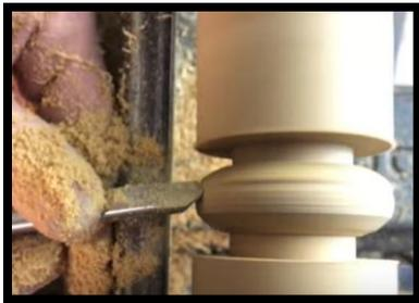
As the name implies, it is designed to perform some of the functions of a skew chisel (with a reduced chance of catches) and a spindle gouge. It can be used to cut beads, coves, v-grooves, and the like (left).
