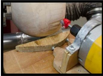
However, when fluting a convex surface such as the outside of a bowl, it requires one to make a custom curved fence (left) which matches the outside of the turning which can be a pain.
