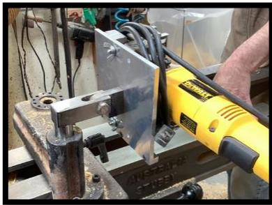
To overcome this limitation, Mike Neal designed a unique jig to hold the joiner (left). It consists of a platform to which the joiner is bolted and a post for mounting in the banjo. A flange on the bottom of the platform bolted to a U-form mounted on the post allows one to adjust the vertical angle of the slot.
