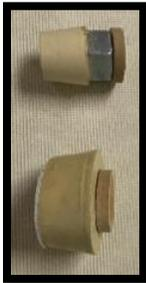
If your live centre does not have a cone or similar fitting for securing a turning without marking the surface, you might want to consider making this jig.
