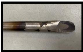
His solution was to use a "fluteless gouge" to make a half-round scraper. The tool consists of an end mill welded to a length of stainless-steel rod. The matching ends were beveled about 1/8" deep, lined up in a long narrow vee block and welded together before being ground to the final dimensions.
