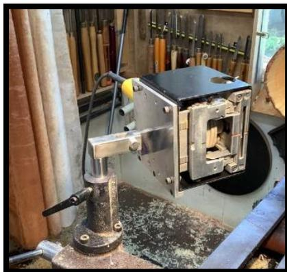
Tim indicated that while it is very versatile when working on a hollow form, the fence on the joiner does impose some limitations if trying to make a slot near the bottom of the turning (especially on a bowl), and the chuck. Accordingly, Mike modified the original version by adding a top mounting plate which allows the joiner to be reversed, thereby providing greater access (left).
