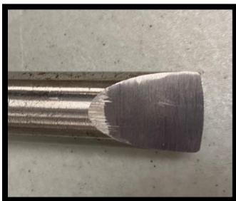
Adam also made these gouges for finishing flats and transitions on platters. They have a slight radius at the cutting edge and, taking inspiration from the *Skewchigouge*, the top is ground to a flat 20 degrees.
