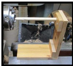
He lines up the end of the dowel with the face of the chuck jaws and marks the position of the jig with masking tape on the ways.
