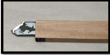
This simple tool consists of a reciprocating saw blade epoxied between two wooden strips. It is useful for cutting fine grooves for decoration or burning.
