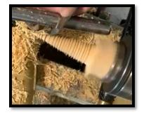
Once the outside shape is formed, "branches" are added using the tip of a skew on an angled cut which produces a raised "fuzzy ring".
