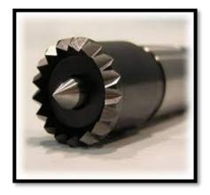
Accordingly, Barrie prefers to use steb centres (left). The centre points are spring loaded which means that as pressure is applied, the point will retract, and the serrated ring will engage the wood.
