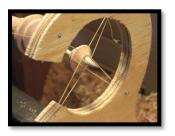
However, as the turning proceeds, it becomes necessary to provide support at the narrow spindle areas. For this purpose, a set of string steady rests are required in which the piece is stabilised by string as opposed to wheels.
