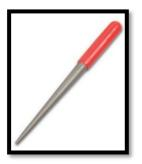
He uses a tapered insert tool (Penn State Industries (PSI): US\$11) which will work with tubes from 7mm to 37/64". (You could also use a 7mm bolt or a turned wooden tool). A twisting motion ensures that the glue is spread evenly, and the tube should be seated just below the surface of the blank.
