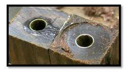
Steve uses a pen mill pilot shaft with a cutter head (aka barrel trimmer) mounted in a Jacobs chuck on his lathe. Alternatively, you could use the trimmer in a drill press or even a drill and a vise. He stated that you should drill slowly and stop when you reach the tube becomes shiny as indicated in the blank on the right in the photo.
