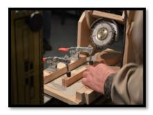
The jig consisted of a 4" angle grinder mounted to a "swing" arm inside a plywood frame. The blank was secured on the platform with two toggle clamps and the angle grinder was rotated in a swinging motion to carve out the bowl portion. While he normally used a chainsaw blade in the grinder, he also has an Arbortech cutter which he uses to make smaller spoons.
